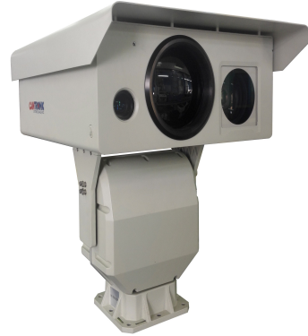
Picture shown camera with pan/tilt and laser illuminator
